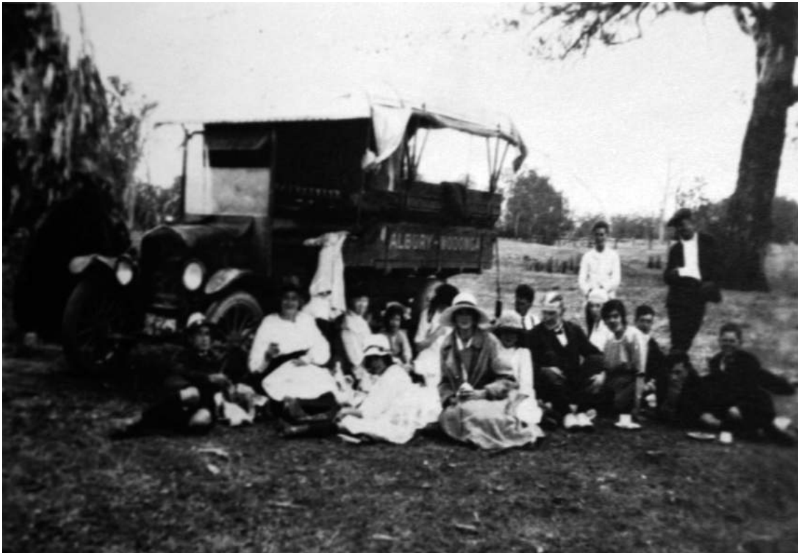
Mylon Motors' first T-Model Ford 15-seat passenger bus. The body was built by Blacklocks. Date of photograph unknown
